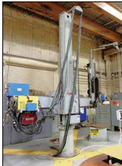
ARONSON WELDING MANIPULATOR SYSTEM
