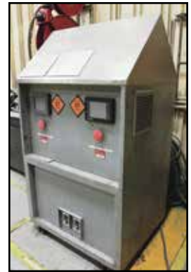
PDS-BARTECH 30.1343 INDUCTION HEATER SYSTEM
